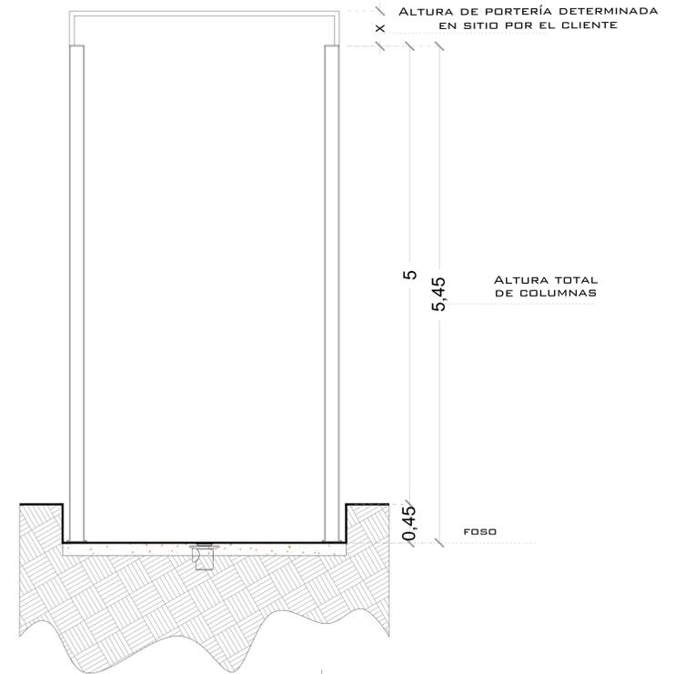
**ALTURA DE COLUMNAS CARGA**
