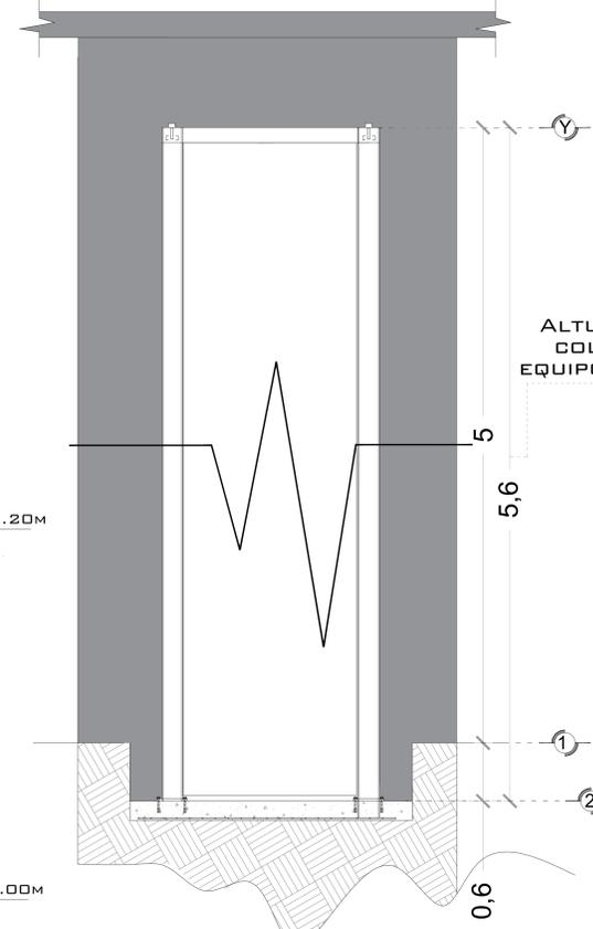
ALTURA TOTAL DE COLUMNAS DEL EQUIPO TECNORAMPA
