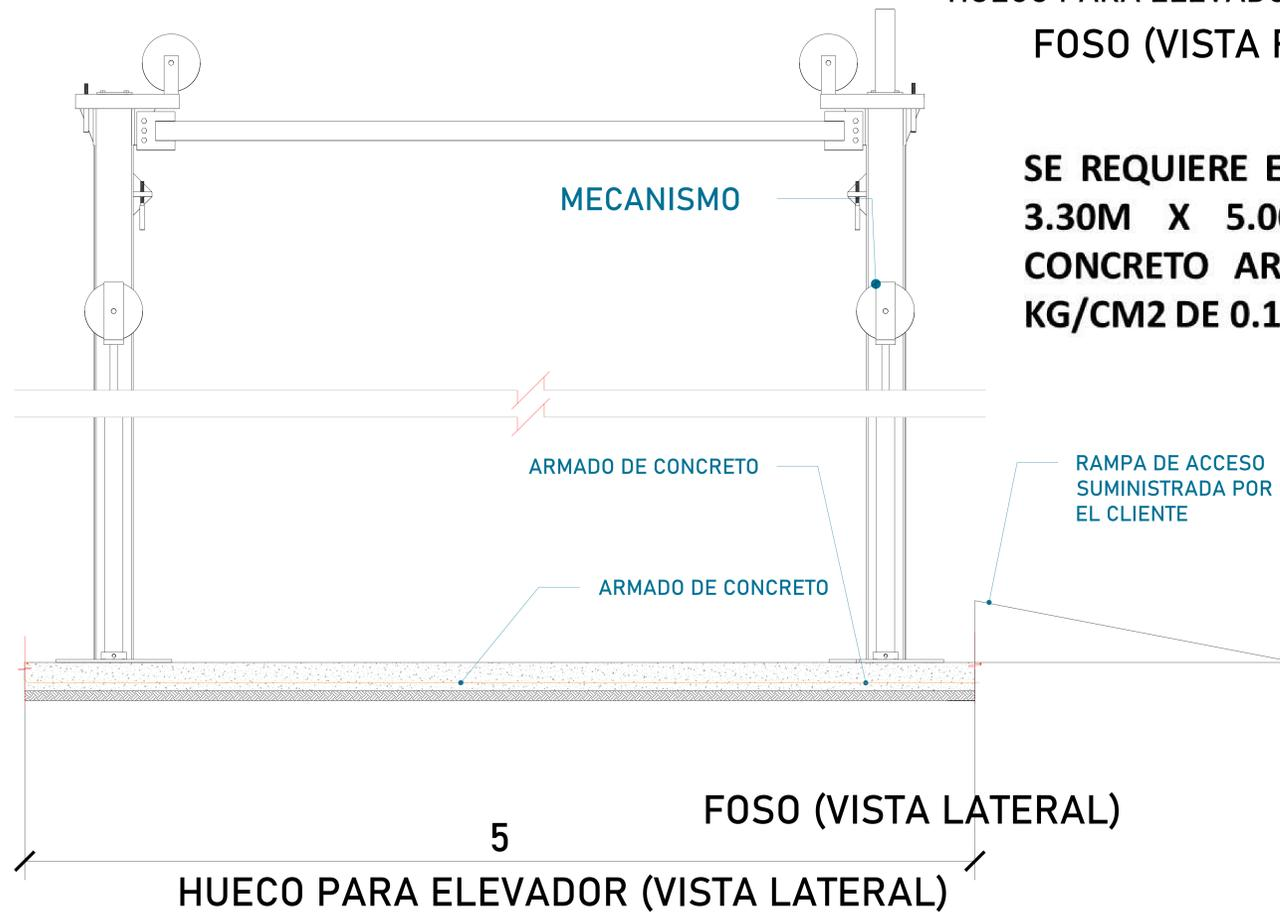
SE REQUIERE EN TODA EL ÁREA DE 3.30M X 5.00M UN FIRME DE CONCRETO ARMADO DE F´C= 250 KG/CM2 DE 0.15M DE ESPESOR
