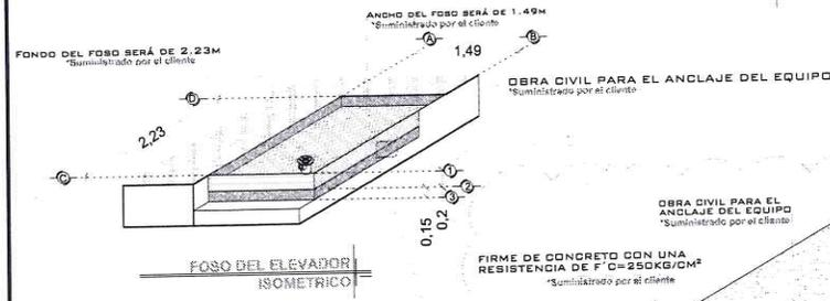
FIRME DE CONCRETO CON UNA RESISTENCIA DE  $F'c = 250 \text{ KG/CM}^2$
