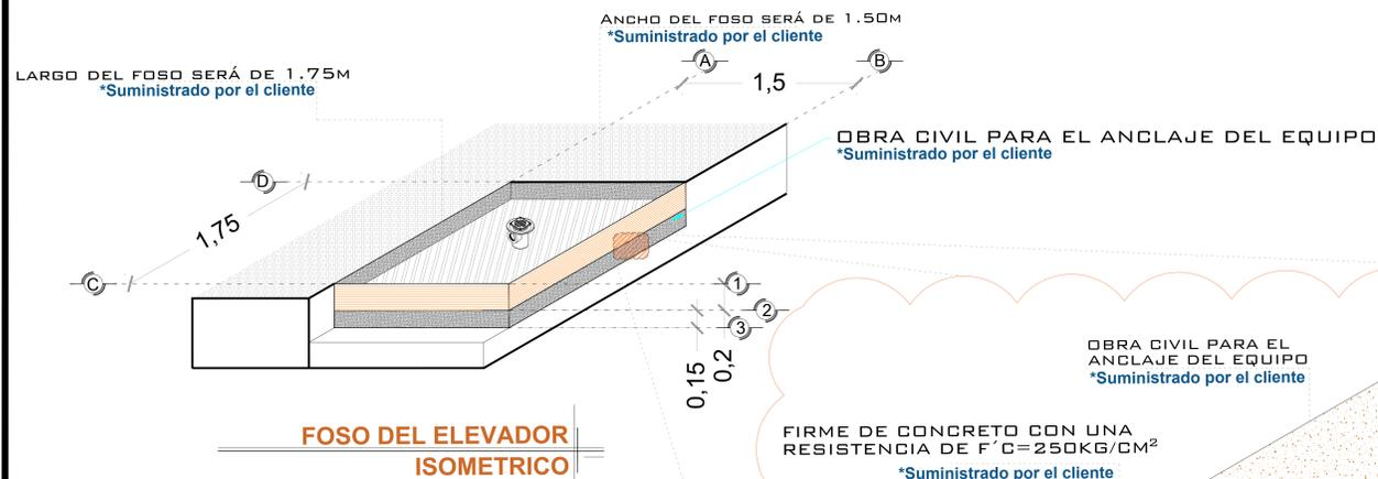
FIRME DE CONCRETO CON UNA RESISTENCIA DE  $F'c = 250 \text{KG/CM}^2$
